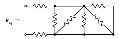
Each resistor is 25  $\Omega$ . Determine the value of  $R_{eq}$ .
